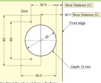
Use Size 5 Countersunk Screws for fixing.
